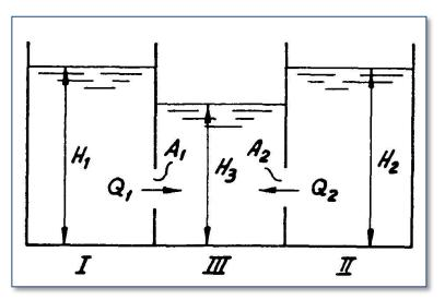
pressures =  $H_1$  and  $H_2$  exist. Through openings with areas  $A_1$  and  $A_2$  respectively the flow  $Q_1$  and  $Q_2$  enter the vessel III, representing the outlet with pressure =  $H_3$ .
