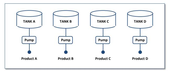
Tanks, including pumps and piping, represent large investments. If it was possible to install a blending unit at the distribution terminal only tanks for the base grades would be needed and for each intermediate grade distributed, one tank with piping could be saved.
