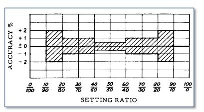
it is not recommended to go beyond these values. Accuracy can be improved by adjusting the inlet pressures, outside the blending unit, in such a way that the diaphragm will stay in centre position (observed on an indicator furnished on request with the unit).
